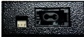
Fig.2. Connectors "Power" and "MOST"
