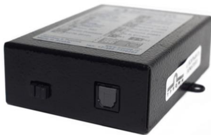
Fig.1. Adapter MOST-TosLink (jumpers and connector "TosLink")
